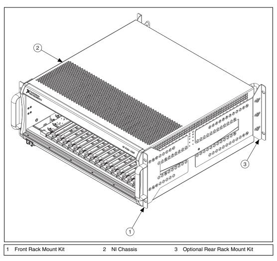
Figure A-3 shows the chassis rack mount kit components.
